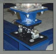
**Four Load Cell scale system** is NTEP Certified. Heavy-duty, 6-inch steel I-Beam frame.
