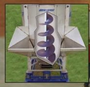
Tapered, 40-inch to 22-inch diameter auger provides thorough, fast and consistently accurate blends. Hopper is 8 feet wide.
